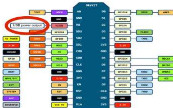
Gambar 2.9 pin NodeMCU Devkit v3[20]
