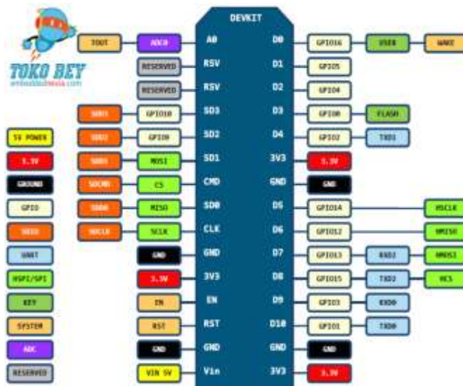
Gambar 2.4 pin NodeMCU Devkit v2[20]
