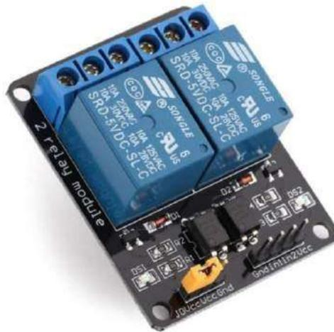
**Gambar 2.6 Relay 2 channel [16]**
