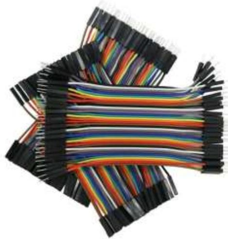
**Gambar 2.8 Kabel *Jumper* Arduino [17]**
