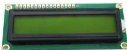
**Gambar 2.12 LCD 16X2 [23]**
