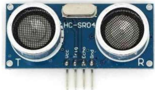
**Gambar 2.5 Sensor Ultrasonik SR04 [19]**
