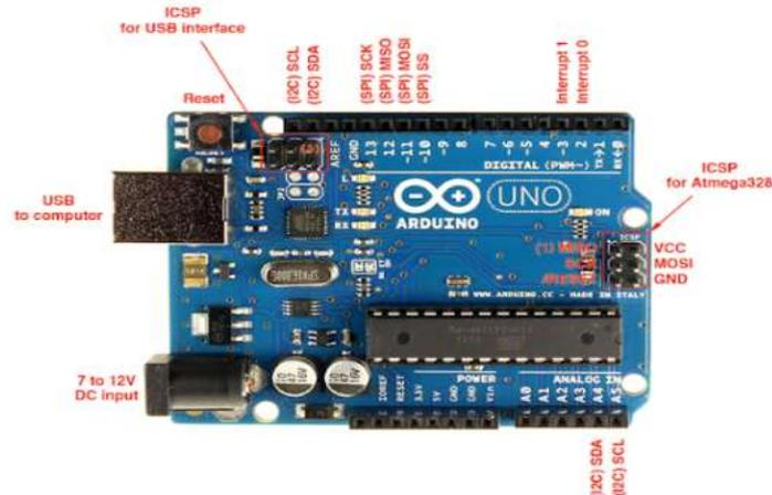
**Gambar 2.2 Pinout arduino atmega328 [19]**
