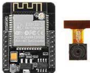
**Gambar 2.7 Esp32-cam [25]**
