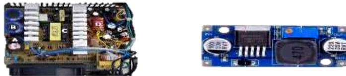
**Gambar 2.9** Adaptor dan *buck converter* dc to dc LM2596 [29], [30]
