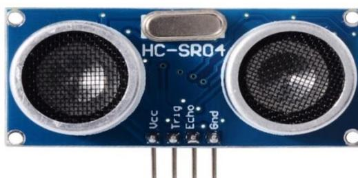
**Gambar 2.12** Sensor *Ultrasonic* HC-SR04 [20]
