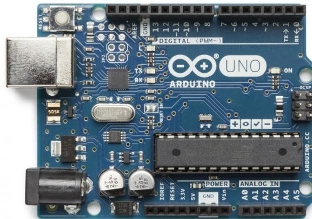
**Gambar 2.16 Modul Arduino uno [21]**
