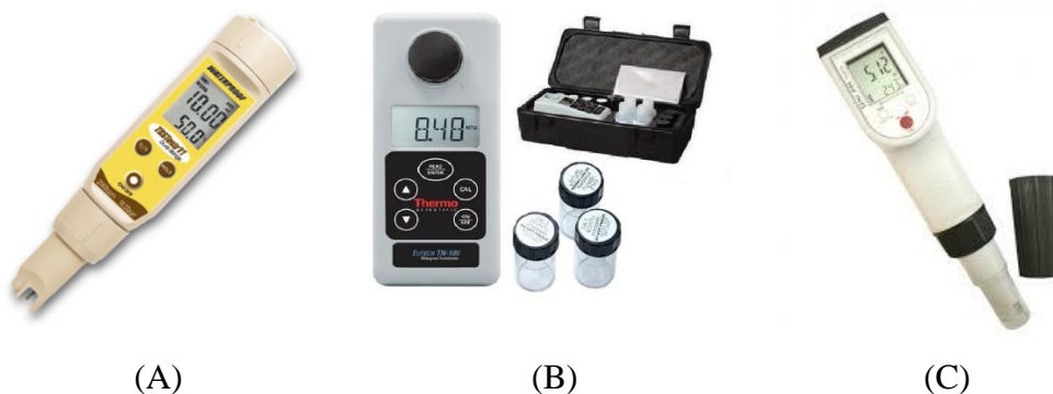
Gambar 3.3 Alat Pengukuran Kualitas Air (A) Eutech TDS Meter (B) Eutech Turbidimeter (C) pH Uni Testa
