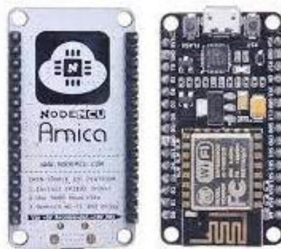
Gambar 2. 12 NodeMCU esp8226 [19]
